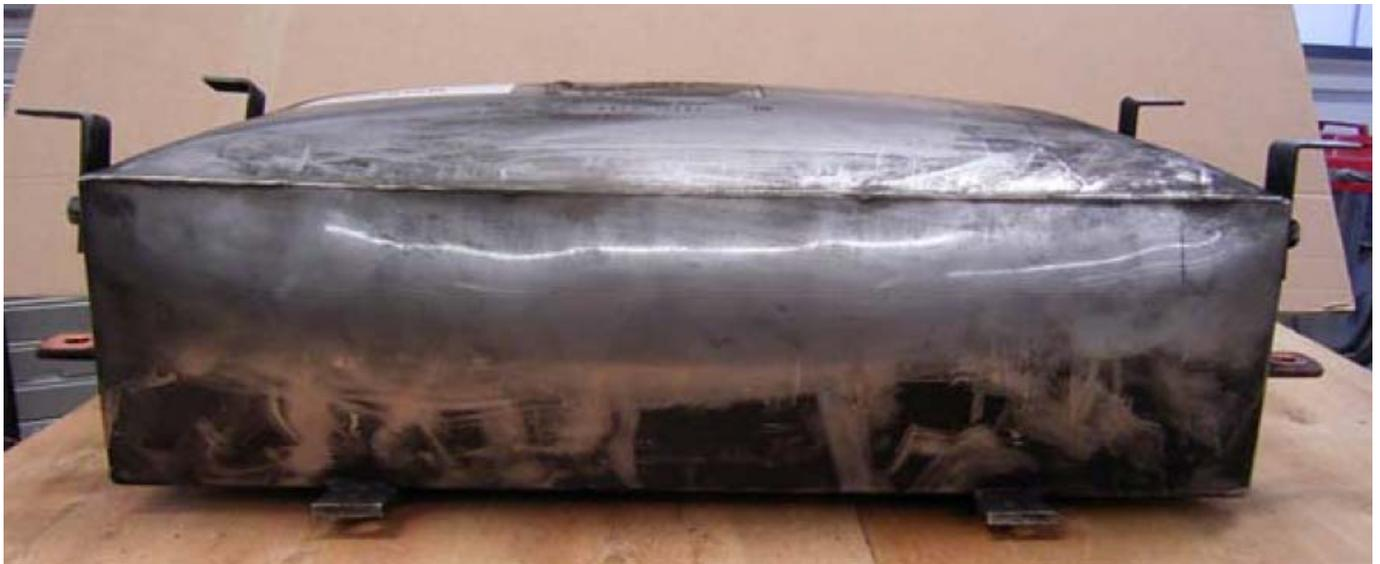
*Picture1. Heavy deformation of RFI filter*
