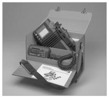
The test instrument, the PSI module, plug inserts, measuring adapter, replacement batteries, recording chart paper etc., can all be conveniently stored and transported with the F100 carrying pouch.
