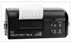
The PSI module is equipped with an RS232 interface, via which stored data can be transmitted at a later point in time to a PC, fully independently of the test instrument
