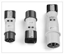
The A3-16, A3-32 and A3-63 three-phase current adapters are used for the convenient connection of test instruments to 5-pole CEE outlets. The three different versions have different sized plugs which correspond to 5-pole CEE outlets with current ratings of 16 A, 32 A and 63 A. Phase sequence is indicated
