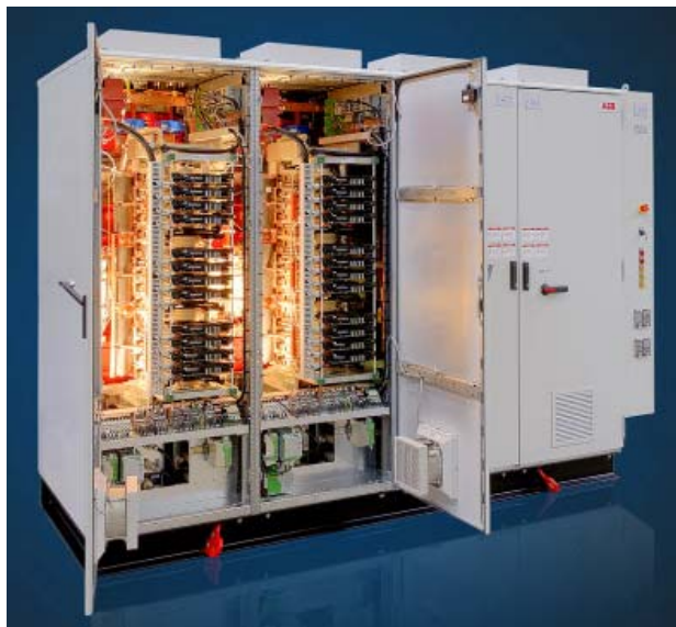
Fig.5. PCS 6000 power cabinet: converter realized using IGCT high density triple stack IGCTs can be exchanged fast and in a convenient way, without disconnecting bus bars or cooling pipes.
