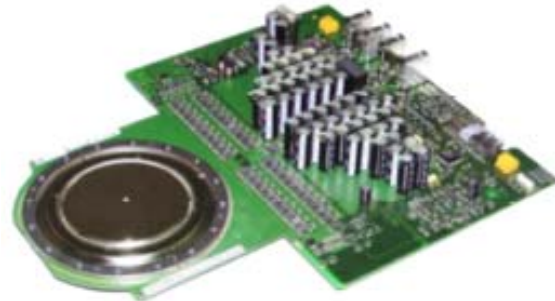
Fig.2. IGCT device used in PCS 6000
