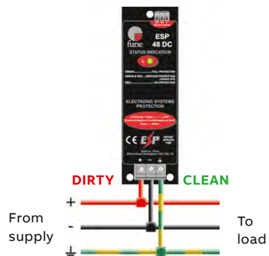
Parallel connection of ESP 48 DC
