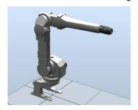
There is also an alternative base for rail mounting of the IRB 5500.
