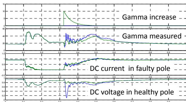
Figure 6, recovery after a DC line fault
