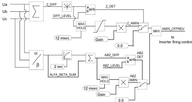
Figure 1, commutation failure prediction, copied from [1]
