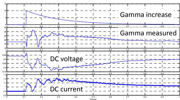
Figure 4, gamma increase at rectifier AC overvoltage
