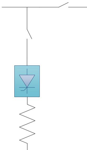
Figure 9, mechanical breaker and thyristor valve in series
