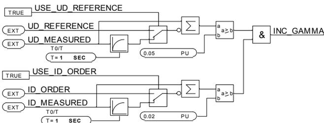
Figure 2, novel commutation failure prediction #1
