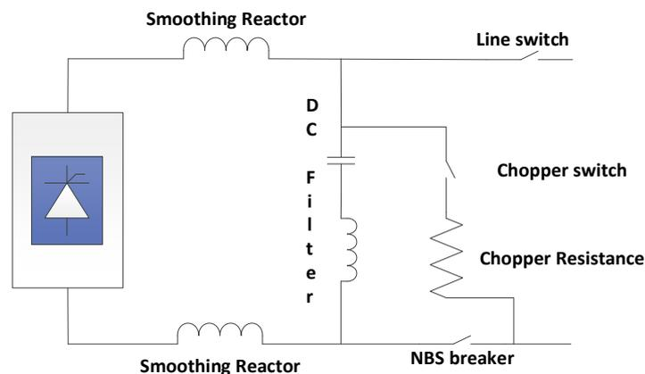
Figure 7, rectifier including DC Chopper
