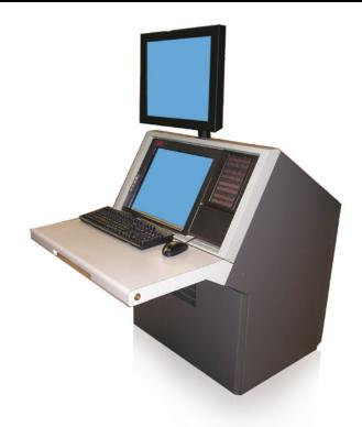
LCD panels need to be able to withstand continuous harsh use, be operational at all times of the day and night, 24x365. An industrial grade LCD touchscreen, is most dependable in harsh industrial environments.
