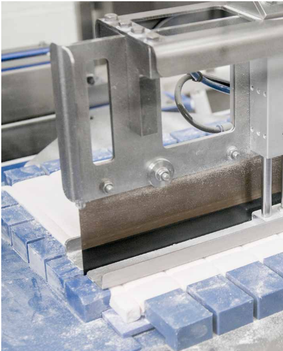
The machines originally cut cakes and sandwiches, but Boomf's IRB 1200 has been adapted to cut personalized marshmallows.
