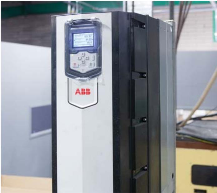
The ABB industrial drive, ACS880, uses the fourth generation motor control platform, direct torque control (DTC), a key benefit of which is highly accurate torque control without encoders.
