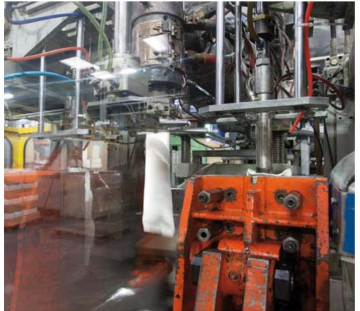
Blow molding requires great precision to ensure product quality and to reduce wastage. Exactly right amount of plastic must be extruded when the mold closes.
