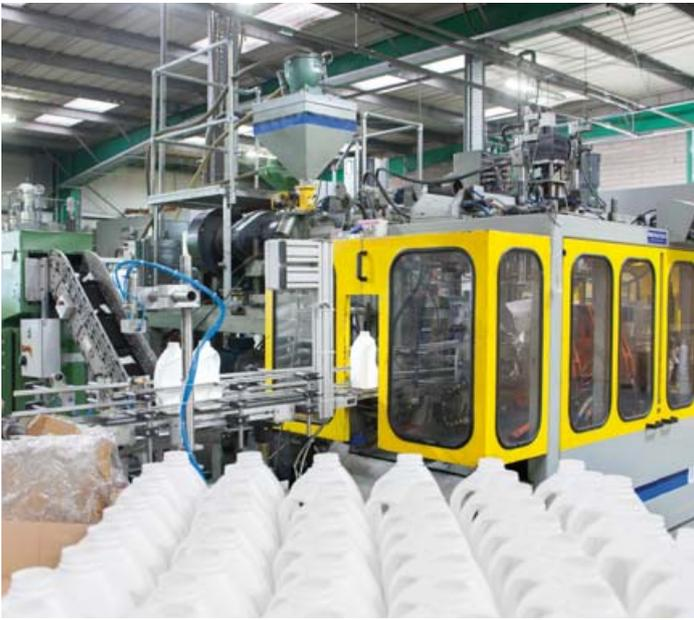
When a 23 year old hydraulic blow molding machine was failing to deliver its proper output, Advantage Control provided the solution. ABB's synchronous reluctance motor (SynRM) and ACS880 variable speed drive package.
