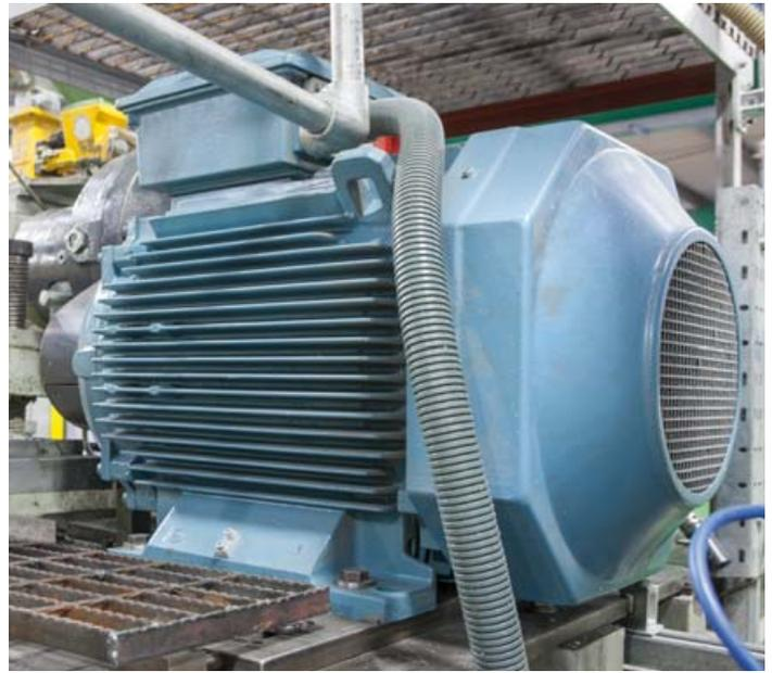
SynRM is running cooler and quieter than the equivalent IE3 induction motor, thus improving the working environment.
