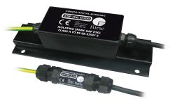
A range of isolating spark gap (ISG) devices (to BS EN/ IEC 62561-3) suitable for equipotential bonding of different earthing systems during transient activity. (BS EN/ IEC 62561-3 supercedes BS EN/ IEC 50164-3)
