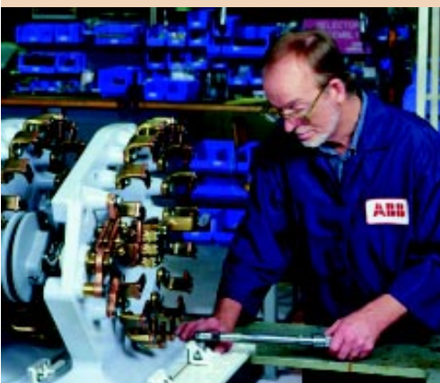
An ABB Technician assembling a Load Tap Changer in the Alamo facility.
