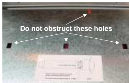
Fuse door cover showing position of striker mechanism slots.
