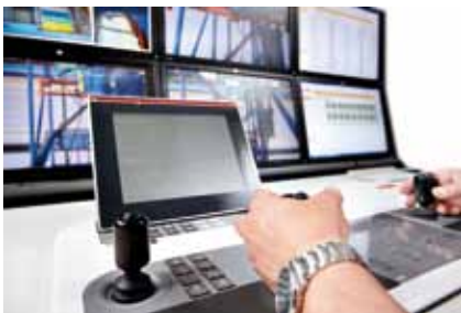
Top: Fast and safe: APS Technology Group's gate automation system at Port of Houston; Below: Control with comfort. ABB's new Remote Control Station for remote monitoring of automatic cranes and handling exceptions.
