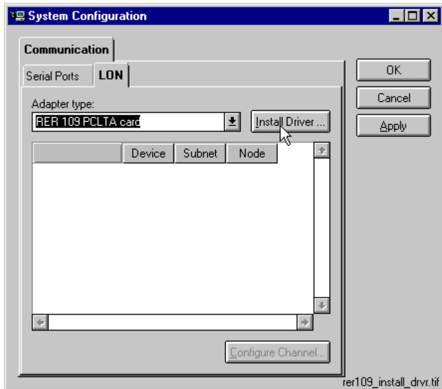
Fig. 4.6.4.3.-1 Starting the driver installation/configuration for the RER 109 PCLTA Card
