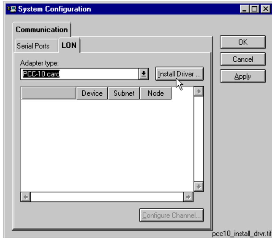
Fig. 4.6.5.1.-1 Starting the driver installation for the PCC-10 PC Card
