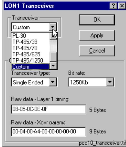
Fig. 4.6.5.2.-2 Switching from the default transceiver setting to the Custom transceiver
