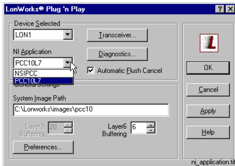
Fig. 4.6.5.2.-1 Selecting the correct NI Application
