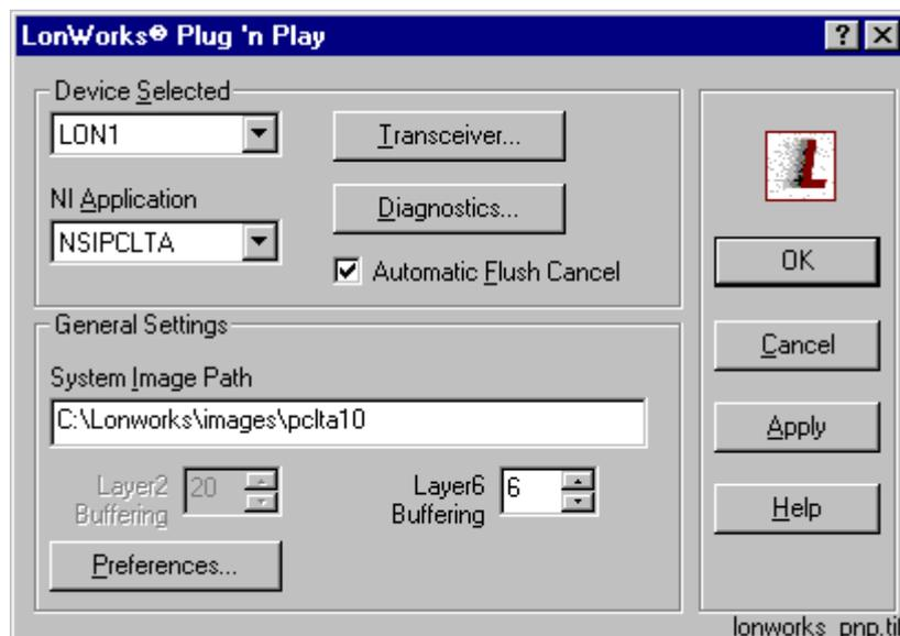
Fig. 4.5.4.7.-3 The LonWorks® Plug'n Play control panel opened for a PCLTA-20 card
