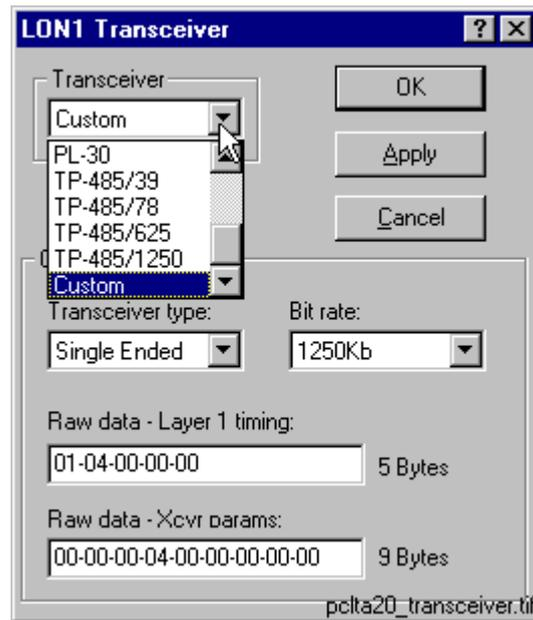
Fig. 4.6.6.2.-3 Switching from the default transceiver setting to the Custom transceiver
