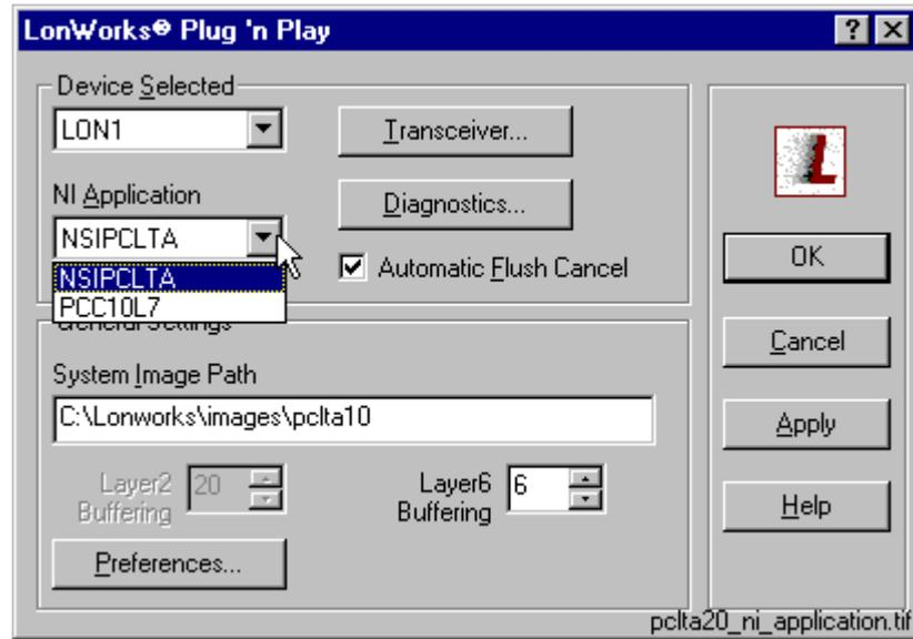
Fig. 4.6.6.2.-2 Selecting the correct NI Application
