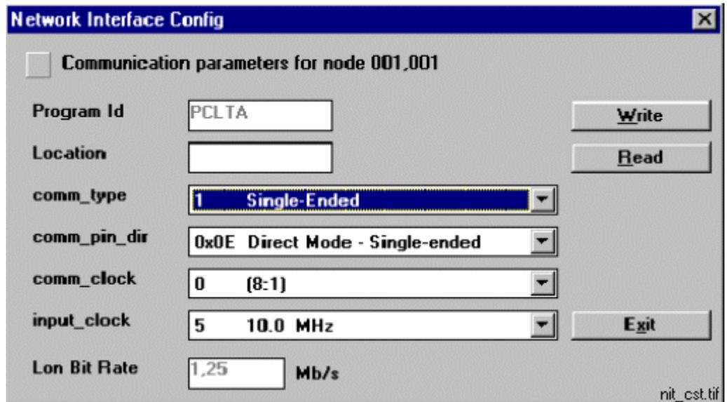
Fig. 4.6.4.5.-6 Sample PCLTA Card Neuron Chip configuration values
