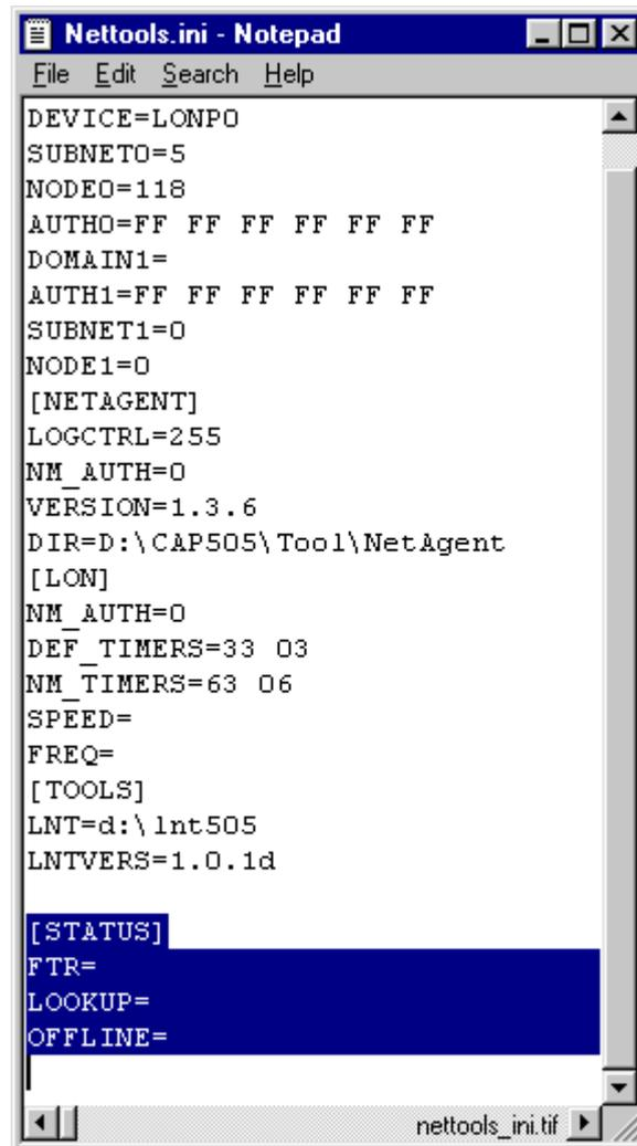
Fig. 4.6.7.3.-1 An example of the file NETTOOLS.INI. As the selection indicates, lengthy data has been written for the critical keys
