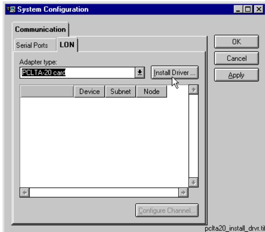
Fig. 4.6.6.1.-1 Starting the driver installation for the PCLTA-20 Card
