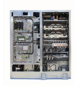
BORDLINE® CC1500 DC converts the power from the 3 kVdc overhead catenary supply into propulsion power required for driving the the traction motors and generates auxiliary power for onboard consumers (AC, integrated battery charger optional).
