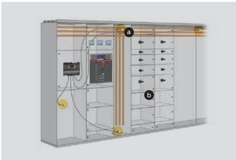
02 a Horizontal and vertical bus bars system b Circuit breaker cubicle
