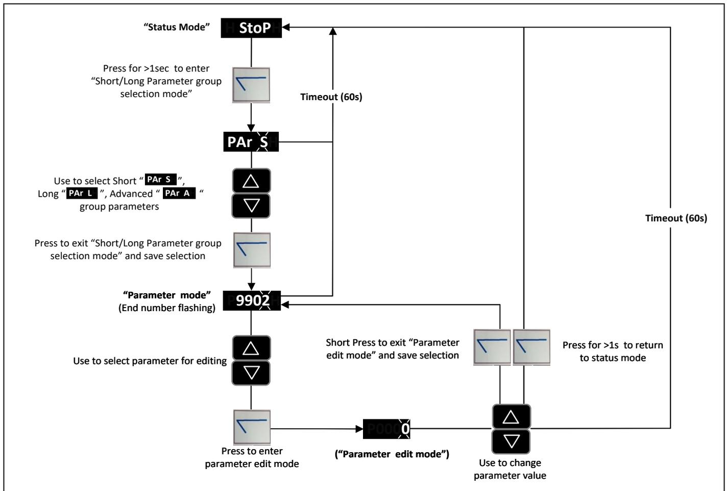
**NOTE** When attempting to edit a parameter the drive must be stopped (not running), if not “L” will be shown on the left side of the display.
