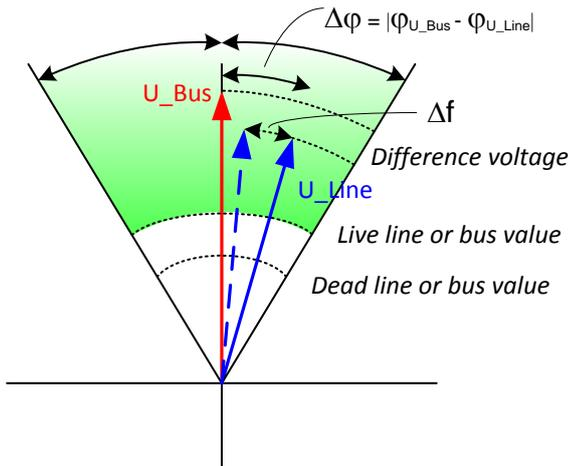
Figure 2. Conditions to be fulfilled when detecting synchronism between systems (phasor diagram)
