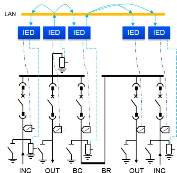
Figure 1. Combined station and process bus
