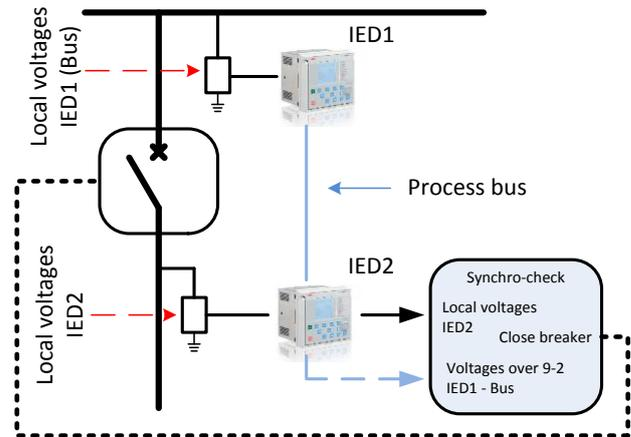
Figure 4. Synchro-check function configuration
