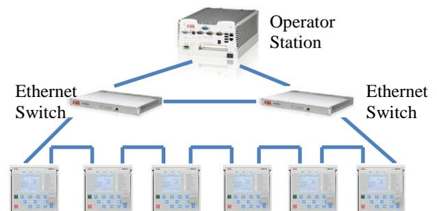
Figure 3. Redundant HSR network
