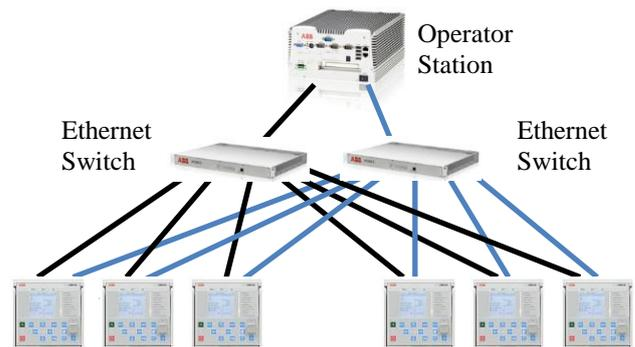
Figure 2. Redundant PRP network.
