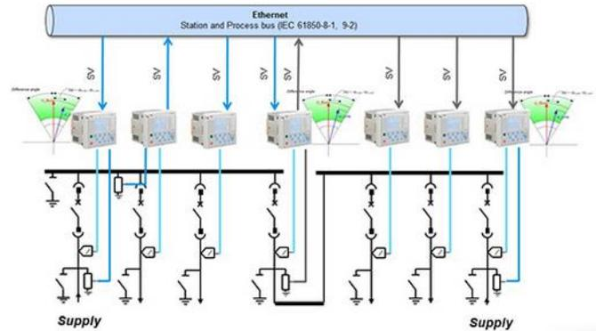
Figure 7. Synchro-check application in switchgear with single busbar arrangement in two bus section arrangement
