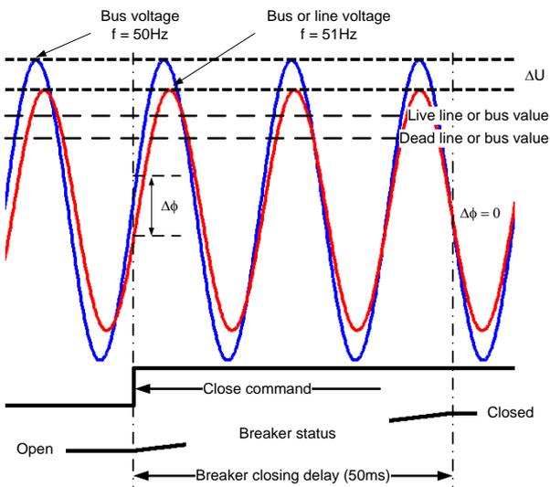
Figure 3. Conditions to be fulfilled when detecting synchronism between systems (time domain)
