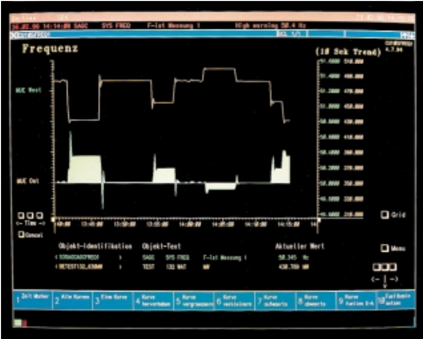
An abrupt change in the power system load (top curve) in isolated operation causes a corresponding reduction in the power system frequency (bottom curve). Without load-frequency control there would be no correction and the frequency would not return to 50 Hz.
