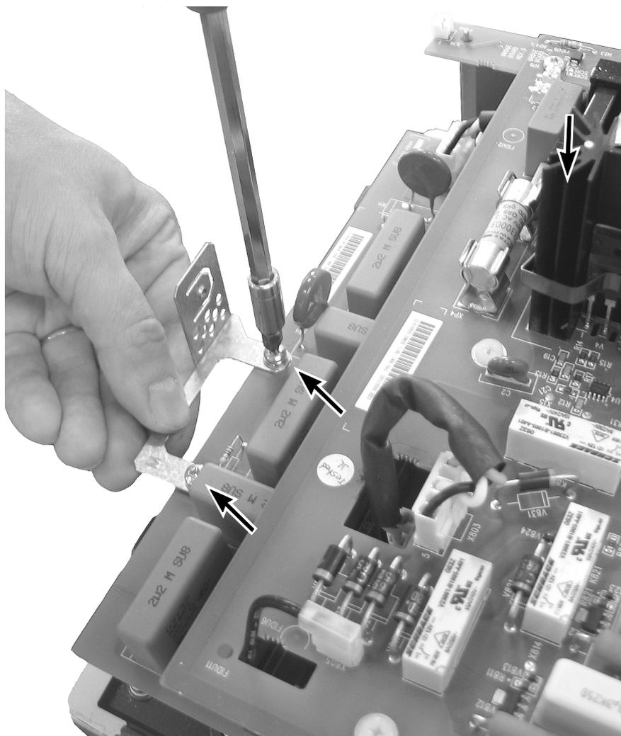
10. Refit the module cover (top edge first) and fasten using the screws removed at step 6. (The screw in the middle of the air outlet grating that was removed at step 5 is no longer needed.)
