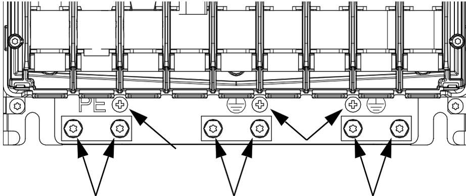
3. Remove the arrowed screws on each side of the module cover. (The middle row of screws is used later to attach the lateral supports of the mounting kit.)
