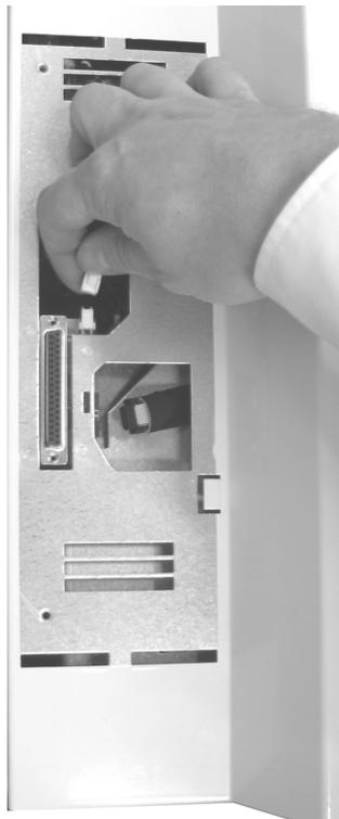
5. Remove the screw in the middle of the air outlet grating.
