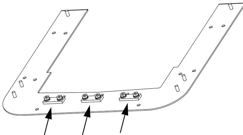
5. Slide the lower collar onto the drive module into the position shown. Fasten through the holes (arrowed) using the three screws removed at step 2.
