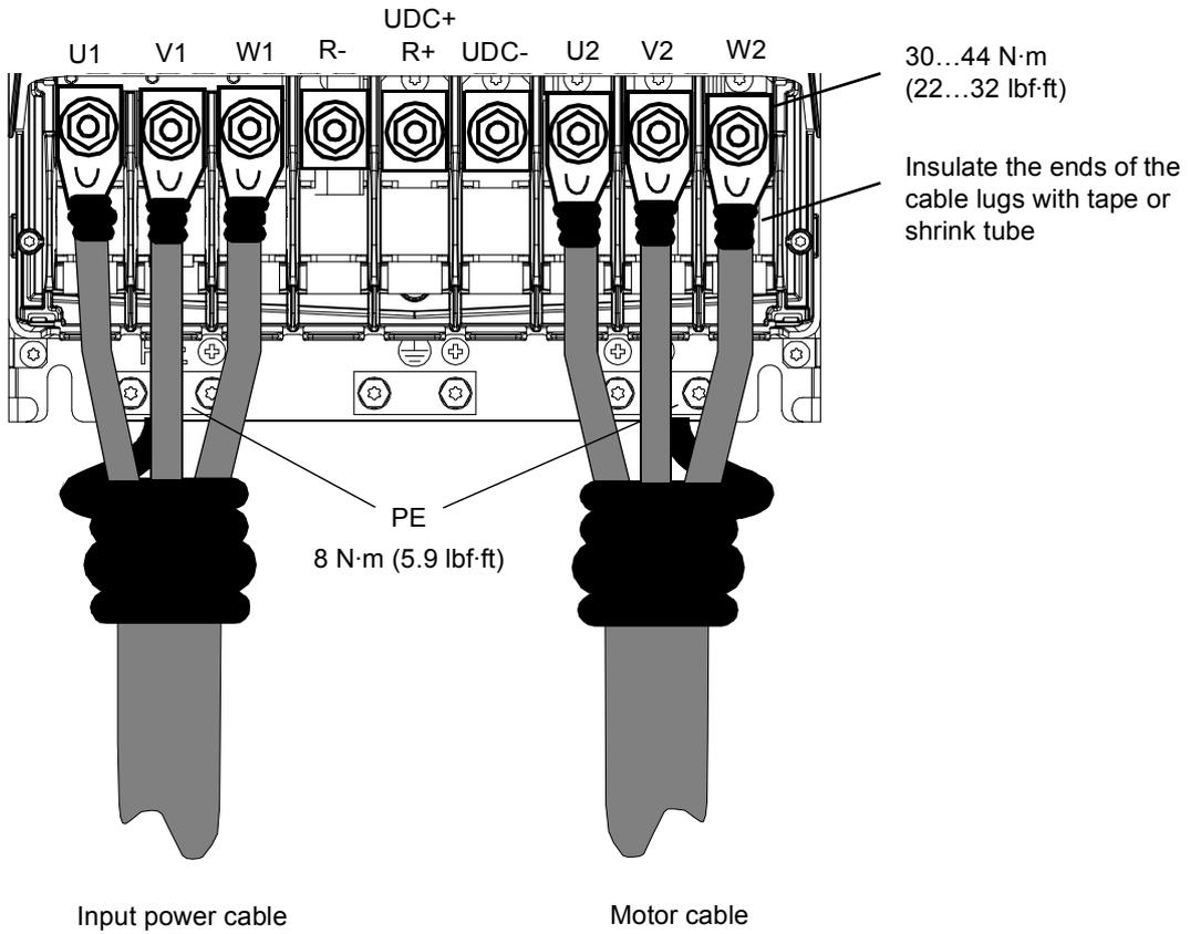
*Screw terminal installation (95 to 185 mm<sup>2</sup> [AWG3/0 to AWG400] cables)*
