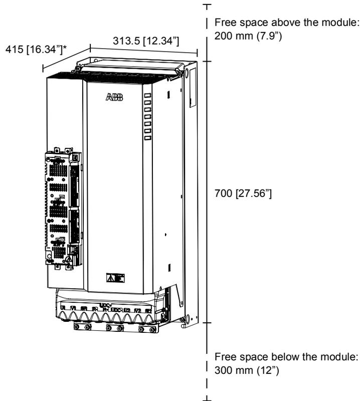
\*Including options installed on the JCU Control Unit. Note that the wiring to some option modules requires approximately 50 mm (2") of additional depth.
