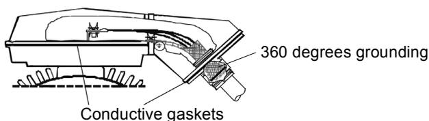
or ground the cable by twisting the shield so that the flattened shield is wider than 1/5 of its length.
