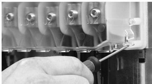
2. Connect the twisted shields of the power cables to the grounding terminals of the drive module.
