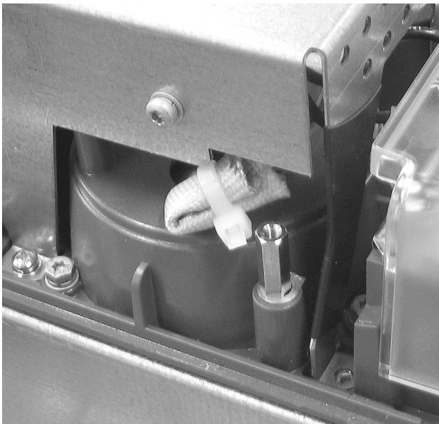
9. Near the top of the module, remove the grounding clip (held by two screws) that connects the varistor board to the module cover.
