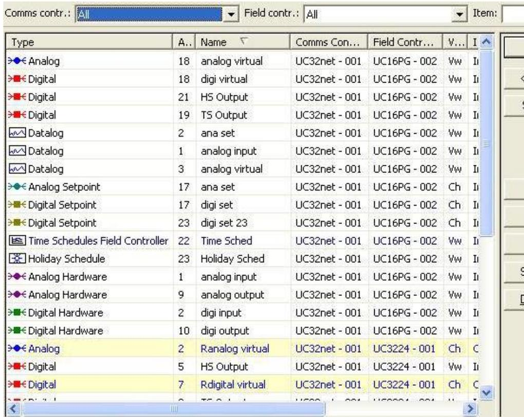
If the keypad is attached to a Comms controller, the database grid can show items from any controller on the site. If the keypad is attached to a stand-alone Field Controller, the database grid will show only items from that Field Controller.
