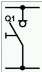
Switch-disconnector bus coupler
