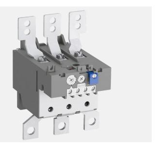
ABB's TA200DU thermal overload relays are economic electromechanical protection devices for the main circuit. They are used mainly to protect motors against overload and phase failures. Starter combinations are setup together with contactors.
