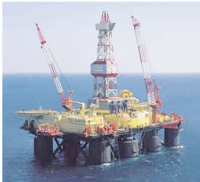
Scarabeo 7 semi-submersible drilling rig
