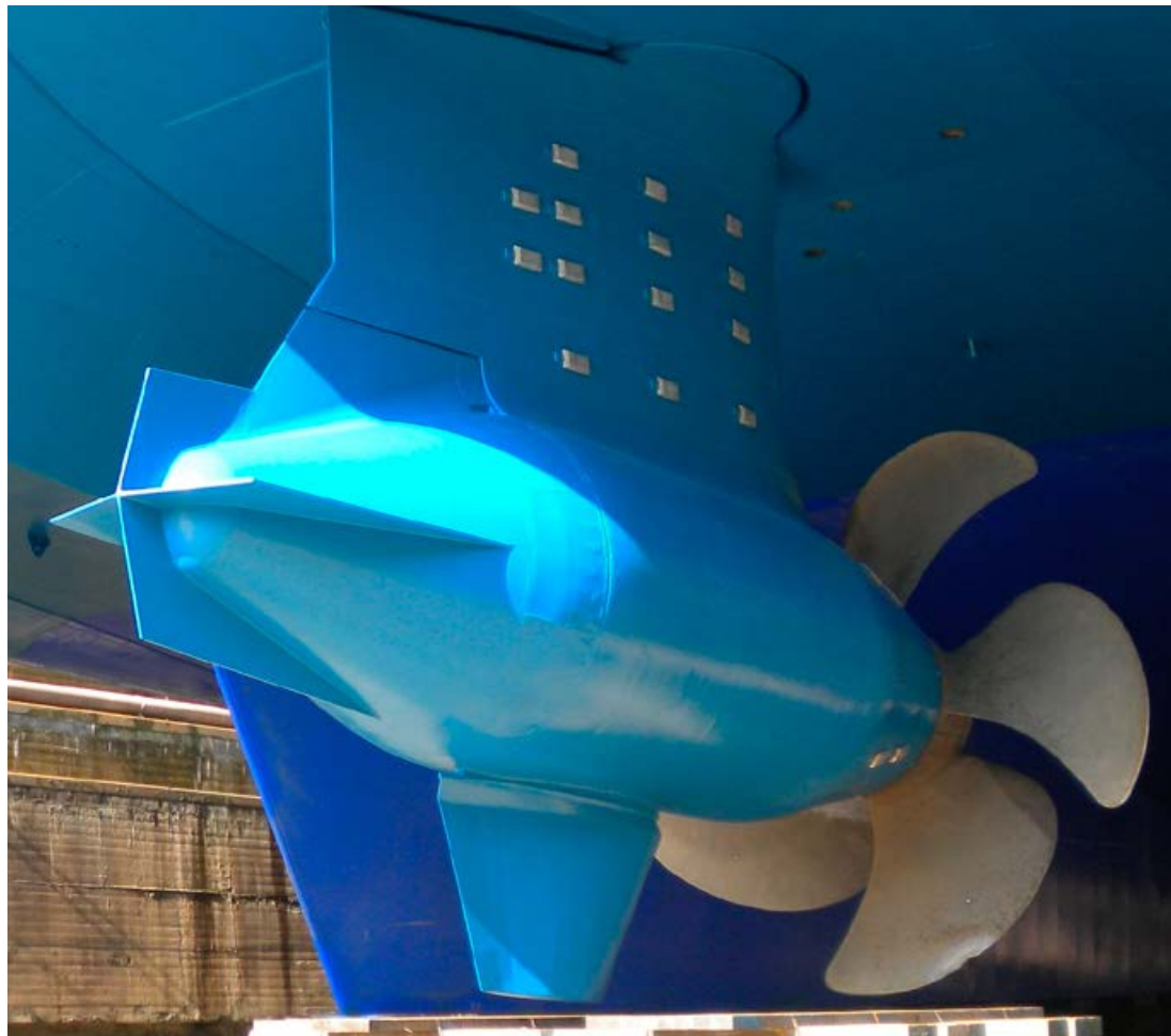
Figure 1: X-tail and asymmetric fin installed during dry docking in 2011. The tests confirmed a 2.8% improvement in efficiency.
