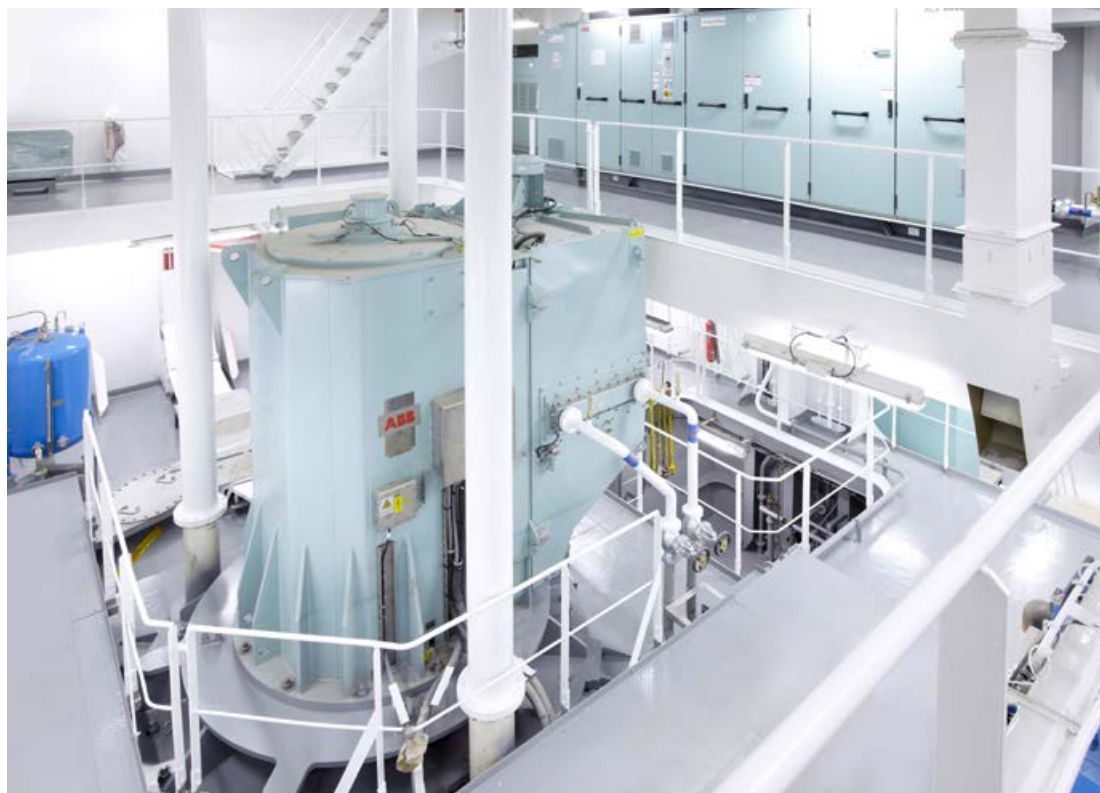
Figure 3: Modular welded frame motor AMI 500 in a thruster application controlled with VFD.
