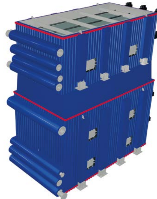
Figure 2: Exhaust gas boiler
