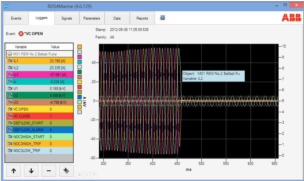
frequency and acquired from REM relays that protect direct on-line induction motors (eg, bow thrusters, pumps, fans) are also used for current spectra analysis to detect mechanical defects of motors such as a broken rotor bar, rotor eccentricity, etc.
