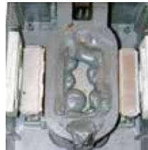
Coil failure. Melted coil due to low voltage condition
