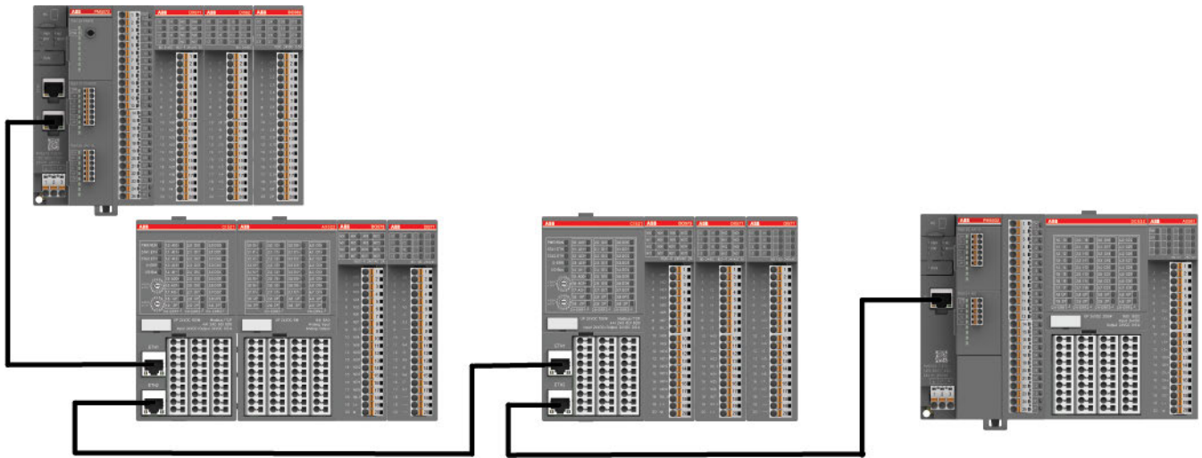
Fig. 4: I/O modules (S500-eCo) connected to an AC500-eCo processor module via Modbus/TCP network, using a Modbus/TCP, PROFINET or EtherCAT communication interface module or a processor module as client.
