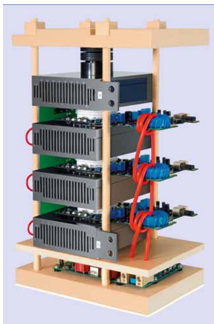
2 Switching unit for the airport radar system
