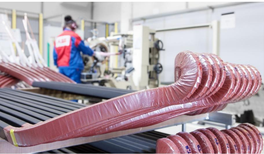
ABB's manufacturing facility located in Beloeil, Quebec, Canada is a world-class manufacturer of hydro generator stator windings. ABB offers both coil and bar manufacturing capabilities to meet our customer's needs.
