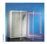
Transparent doors with tempered glass plate (4 mm gauge) secured internally per safety norms. The hinges are not visible from the outside, door opening radius up to 120°.
