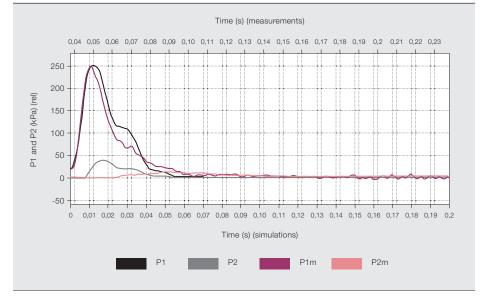
4 Comparison of calculated and measured pressure developments for an internal arc in ZX2 using SF as filling gas (35 kA)
