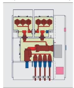
Type tests not only verify that the switchgear enclosure withstands the pressure, but also prove that hot gases are directed away from personnel.
