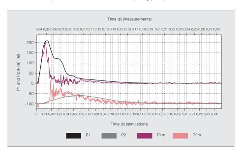
10 s for a maximum arc duration of 1 s on a laptop. The calculations are performed with a constant simulation time step of 0.05 ms. For comparison with tests, measurement data in proper format can be imported.
