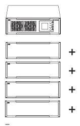
**Up to 4 battery modules can be added** 5 - 10 kVA units
