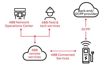
Better and faster support: Chargers connected to ABB's network operations center can achieve the fastest remote support from ABB network engineers. This leads to higher uptime of a charger network, minimizes the number of unplanned on-site visits, and significantly reduces overall operational costs.
