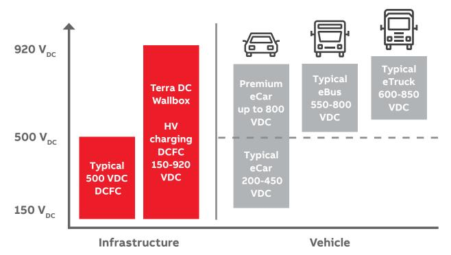
A high range of DC voltage capability is demanded to deliver efficient charging services to every EV and use case.
