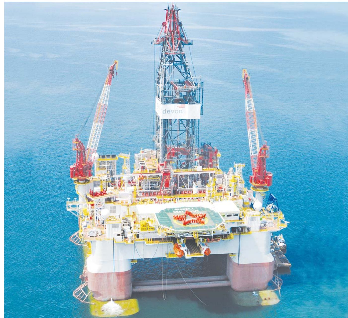
West Sirius was delivered to Seadrill in 2008 from Jurong Shipyard. This 6th generation semi-submersible drilling rig is equipped with Power Generation and Distribution Systems, Thruster Drive Systems and Drilling Drive Systems from ABB.
