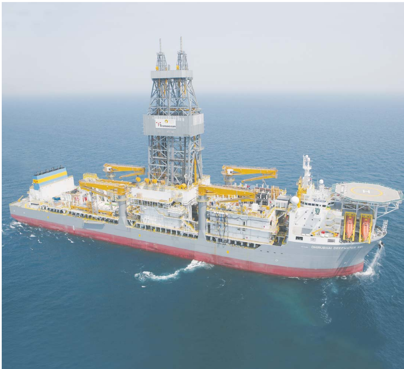
Dhirubhai Deepwater KG1 was delivered to Transocean in 2009 from Samsung Heavy Industries. This advanced deepwater drill ship is equipped with Power Generation and Distribution Systems, Thruster Drive Systems and Drilling Drive Systems from ABB.
