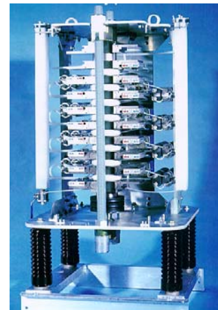
Fig. 6. Thyristor valve of BCT design.
