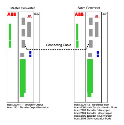
The master converter (Object Index 2230 = 1 - Emulation Output) provides an encoder-emulated output signal. Resolution of this signal can be parameterised using Object Index 2231, Encoder Output Resolution.
