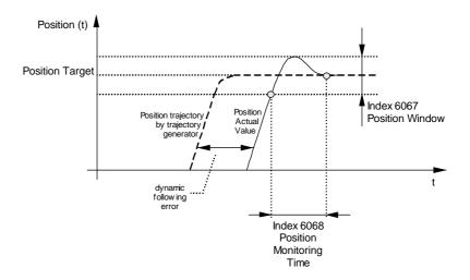
The positioning is successfully completed when the position actual value lies within the Position Window before the Position Monitoring Time expires.
