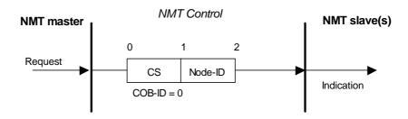
The NMT command specifiers (CS) used for controlling the node are:
