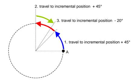
Note that in any case of absolute and relative positioning, approaching direction to the target depends on sign of position setpoint: clockwise rotation when positive setpoint, counterclockwise rotation when negative setpoint.
