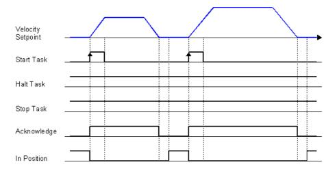
A positive edge of command signal "Start Task" activates a new positioning task; a positive edge of status signal "Acknowledge" indicates that the positioning started.
