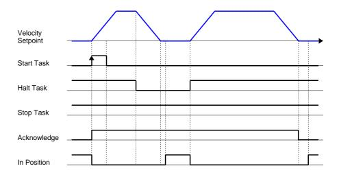
As a command Halt Task is activated, the unit halts the positioning task and sets the signal "In Position". As Halt command is released, the unit restarts and finishes positioning.
