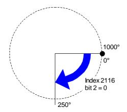
Note that only position targets less or equal to the position modulo are allowed.
