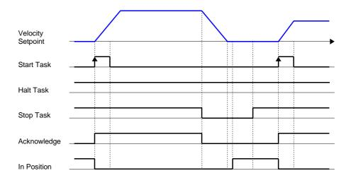
As a command Stop Task is activated, the positioning task is aborted. The unit stops and sets the signal "In Position". As Stop command is released, the unit may be restarted with a new "Start Task" command.
