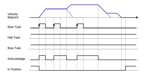
A positive edge of command signal "Start Task" activates a first positioning task; a positive edge of status signal "Acknowledge" indicates that the positioning is being executed.
