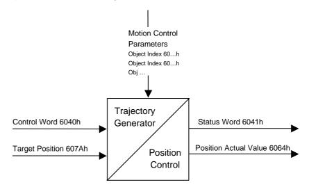
This operating mode of DGV supports various positioning functions for different purposes and applications. A detailed description of these functions is given in the following paragraphs.
