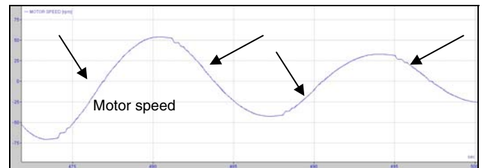
Figure 10. Backlash during coast stop.
