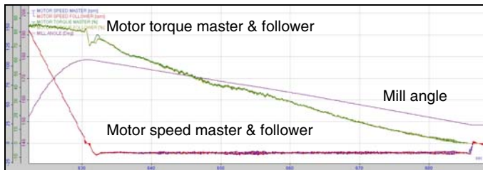
Figure 19. Close up view of controlled rollback (master/follower).
