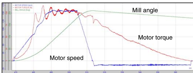
Figure 12. Automatic positioning routine with 180° angle reference.
