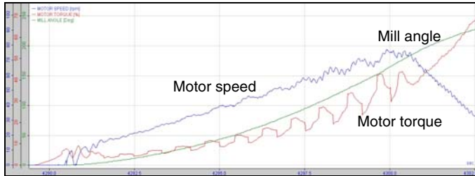
Figure 14. Frozen charge remover torque steps.
