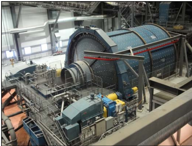
Figure 15. 2 x 5 MW dual pinion ring geared pebble mill.
