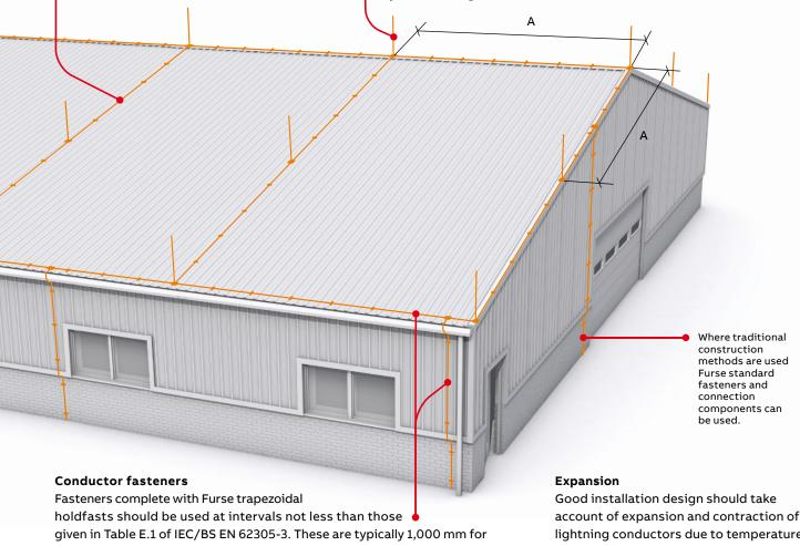
holdfasts should be used at intervals not less than those given in Table E.1 of IEC/BS EN 62305-3. These are typically 1,000 mm for horizontal conductors on horizontal surfaces and 1,000 mm for vertical conductors from ground level up to 20 m high. The use of metallic clips and bare conductor is recommended for air-termination network design to promote effective current sharing across the roof. Non-metallic clips and covered conductors may be used as part of the down-conductor system.
