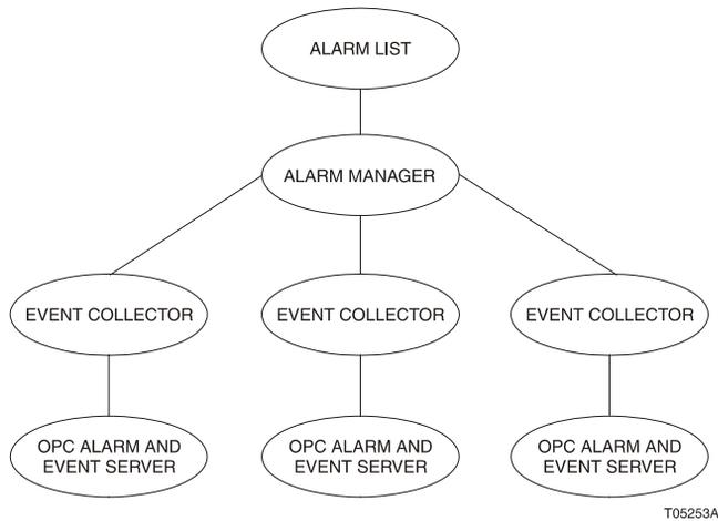
*Figure 11. Alarm Manager and Event Collector Layers for System 800xA 5.0 SP2*
