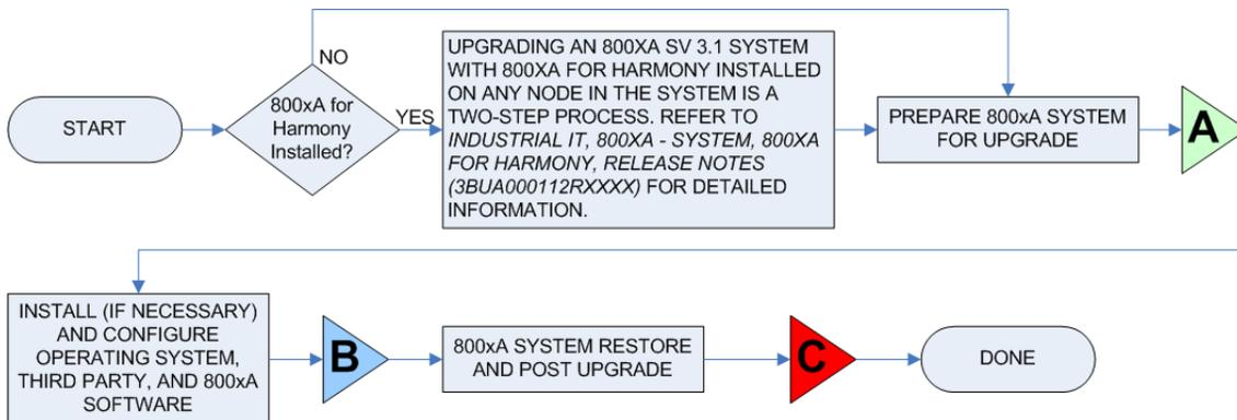
Figure 1. High Level Upgrade Flow
