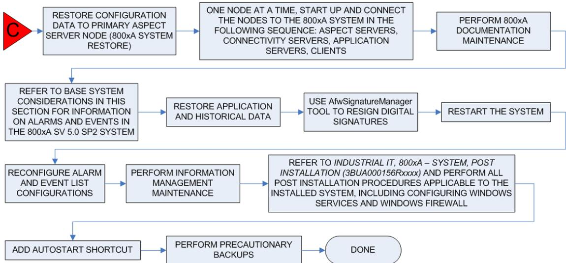
Figure 4. System Restore and Post Upgrade Flow
