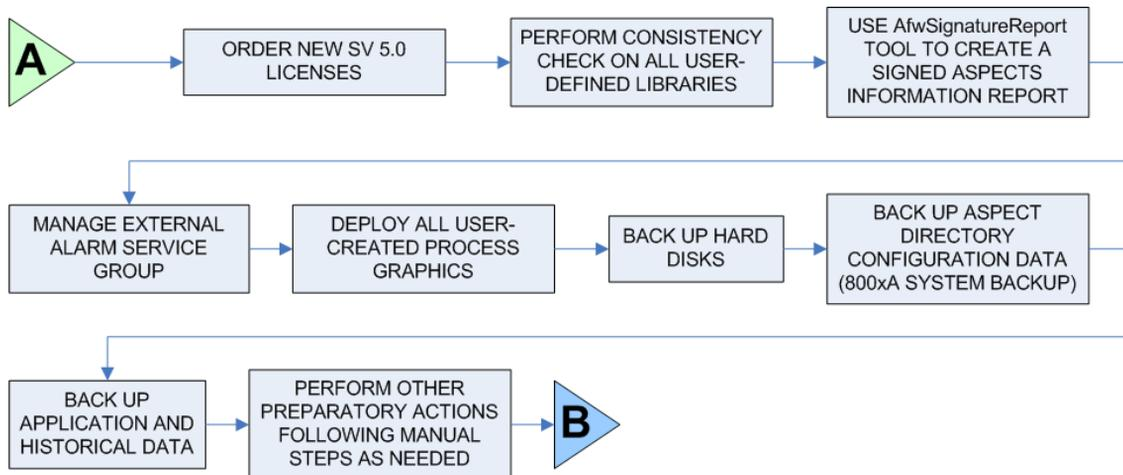
Figure 2. Upgrade Preparation Flow
