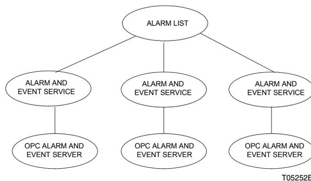
Figure 10. Alarm and Event Service Layer for SV 3.1 SP3
