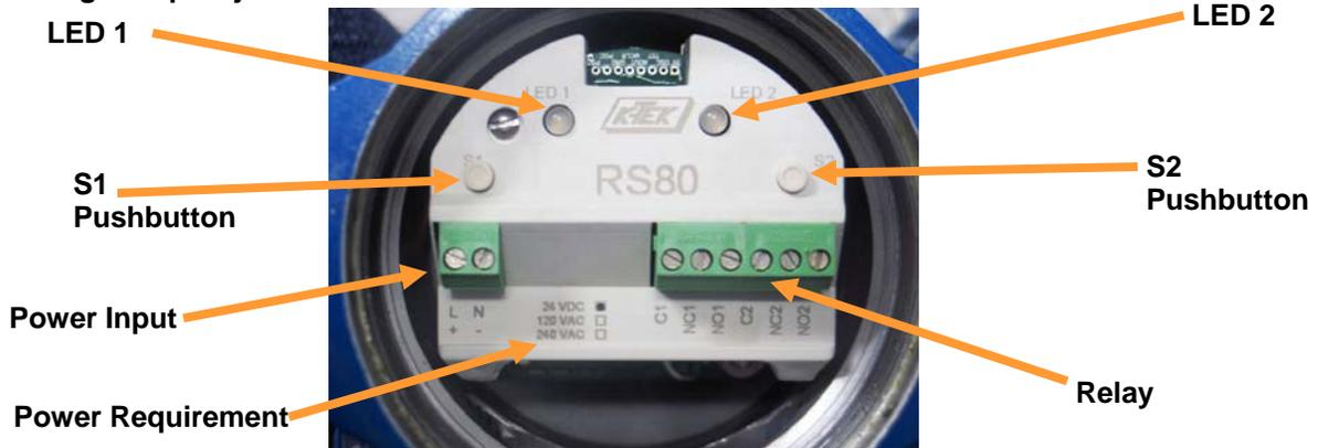
Setup of the Resonator may be achieved using a (1) magnet positioned on the housing or (2) by means of the pushbuttons on the module. In the following operations, pushbuttons will correspond to magnet positions as follows:
