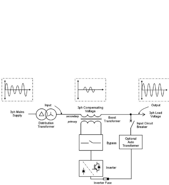
Figure 2: Block diagram of ABB's AVC
