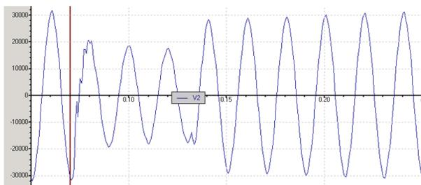
**Figure 1: Voltage dip captured at 22kV**
