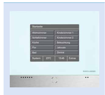
1 The Control Panel serves as central user interface.
