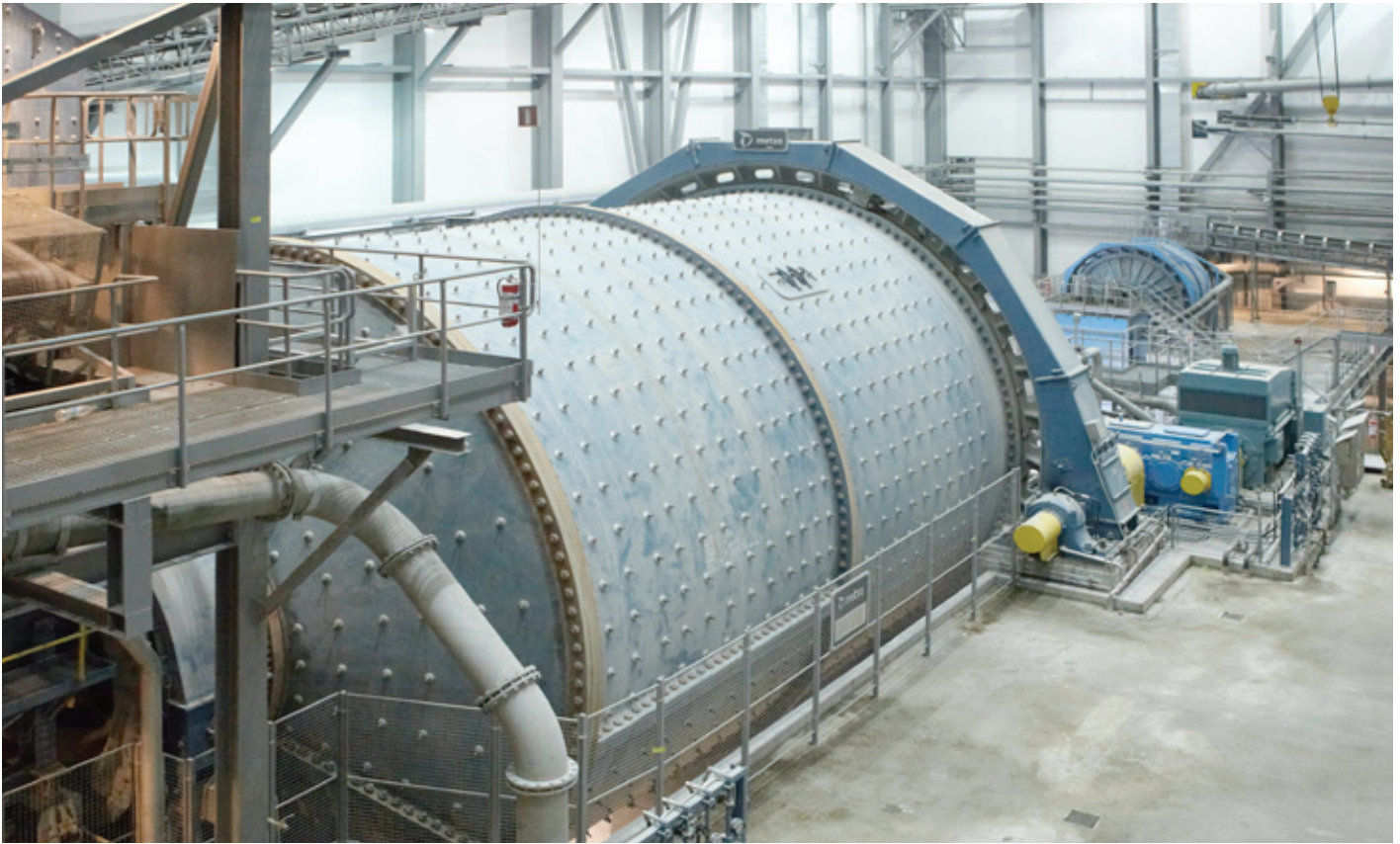
Gearless mill drive at Aitik. The capacity is 2,200 tonnes per hour.
