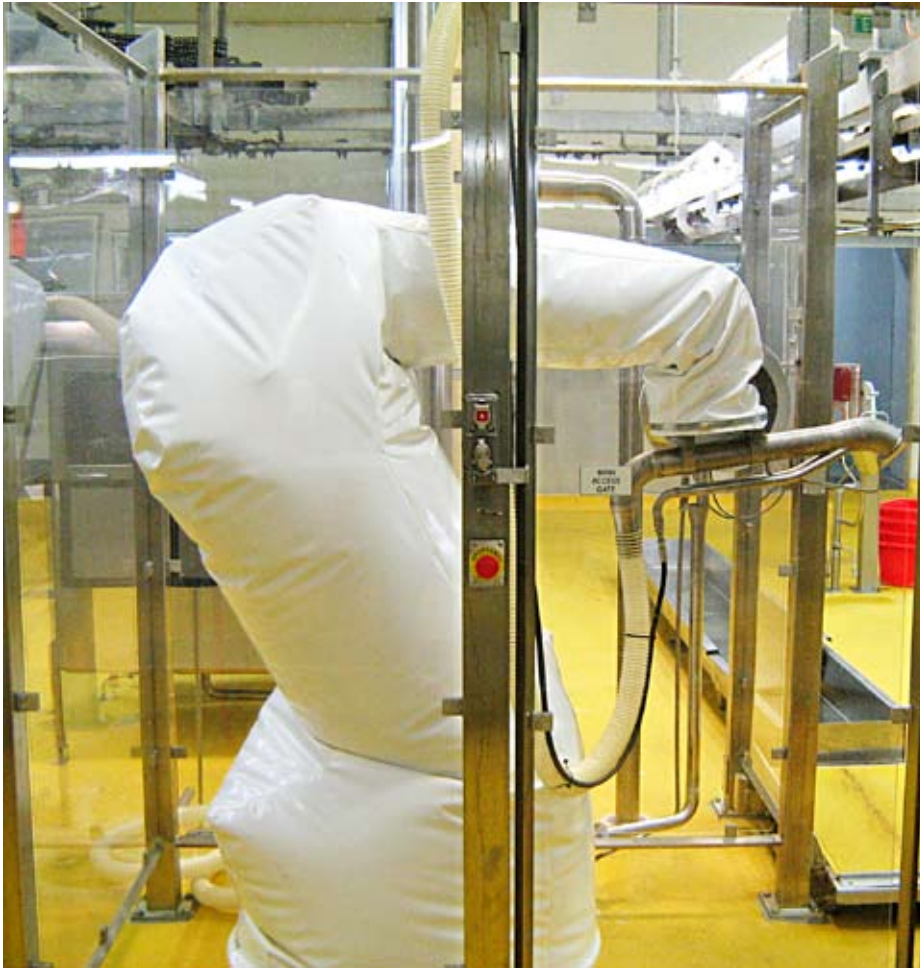
An IRB 4600 industrial robot is fitted with a vacuum wand to remove kidney fat.
