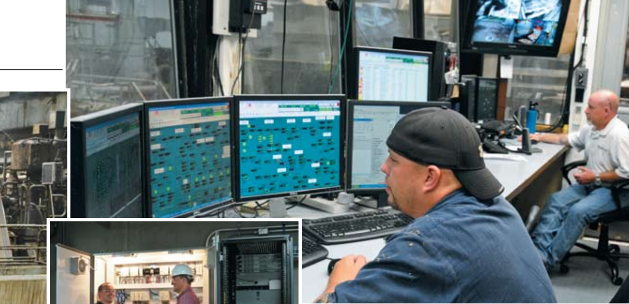
Rand-Whitney's machine and related equipment include about 1,600 I/O connections and about 500 process control components.
