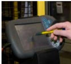
The FlexPendant makes for user-friendly operation of the robots.
