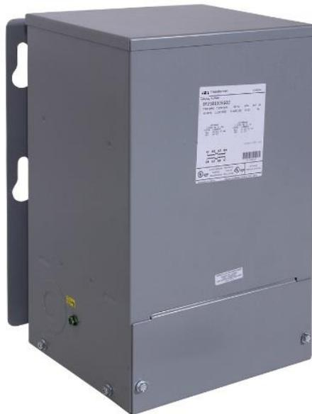
**Fig. 1** Wall mounted, TENV construction with single-phase ratings, 5-25kVa and three-phase ratings, 3-15kVa.
