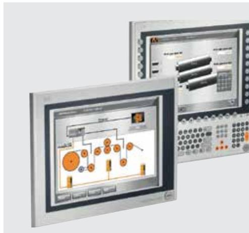
The ABB B&R Automation Panel 900 is an industrial operator interface that fulfills the highest quality demands. In the ABB-tacteo project, the Panel 900 is the default interface for human-machine collaboration on all main production stations.
