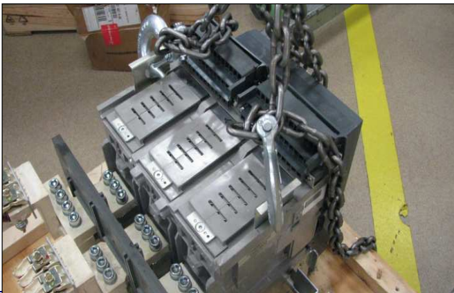
Figure 8. Crane Lifting Hooks Can Damage lifting Ears and Chains Can Damage or Scratch Fascia
